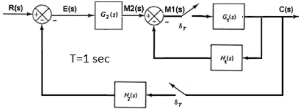
Where  $R(s) = \frac{1}{s}$ ,  $G_1(s) = \frac{K}{s+1}$ ,  $G_2(s) = \frac{s}{s+1}$ ,  $H_1(s) = \frac{5s}{s+1}$ ,  $H_2(s) = \frac{K}{s}$
